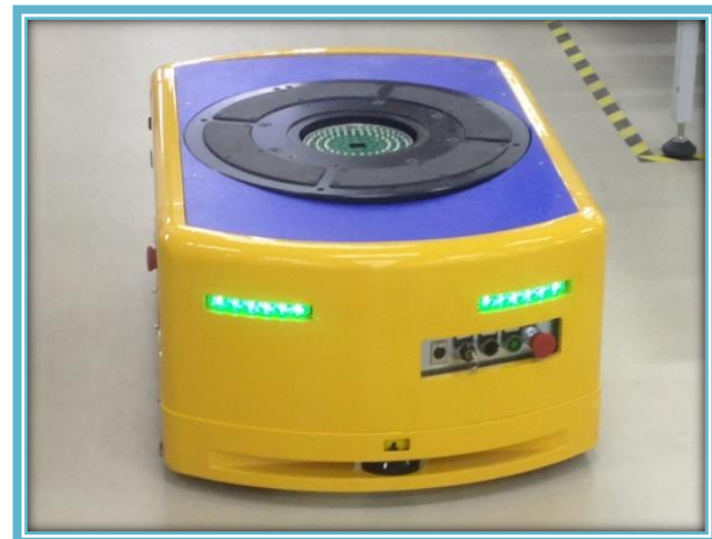
AGC(Autonomous guided cart) Towing capacity = 1000kg
