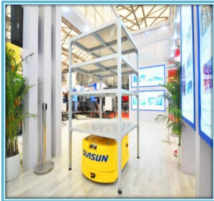
AMR(Autonomous mobile robot) Loading capacity = 500 kg
