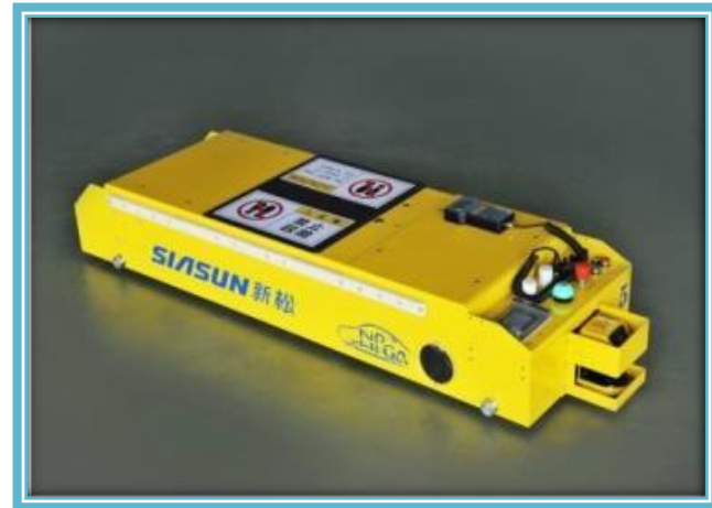
AGC(Autonomous guided cart) Towing capacity = 1000kg
