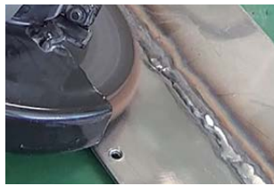
Removing blue weld discoloration
