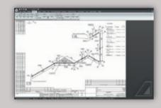
The software can then not only provide a wide variety of different reports, worksheets and documentation for these spools, but also the CNC data for the various machining processes.
